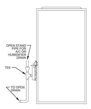
Fig. 49—Example of Field Drain Attachment
